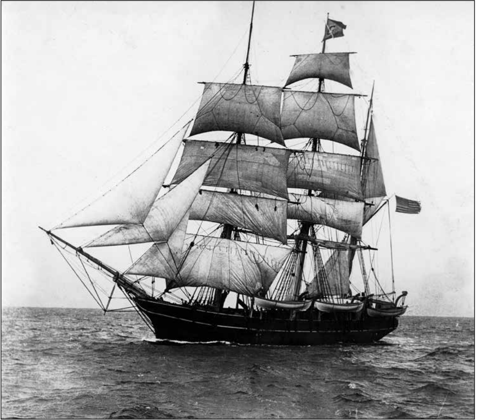
A typical offshore whaling vessel, the bark Swallow ; the tryworks, used to render blubber into oil, would be located behind the foremast. MV Museum Photo Collection, File 1850a.
