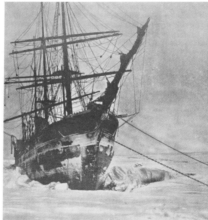
A total loss, America's reinforced bow rests on the ice undamaged, her stern planking crushed and engine room flooded. Midnight photo taken in moonlight.
