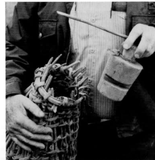
George Manter shows how stakes were driven to keep the beach pot from drifting with the current. Below, wooden plug, held in place by a slender stick, closed the pot's narrow end. No metal was used in the pot.
